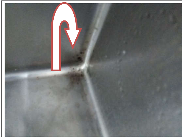
Oxidized in the corner because user leaves the corners too wet with water on the surface for a long time without cleaning it. Oxidation can occur.
